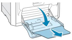
2 Load letterhead only in the Multi-purpose Tray with the print side down and the top, short edge, in first. Adjust the guide to fit the width of the paper stack.
